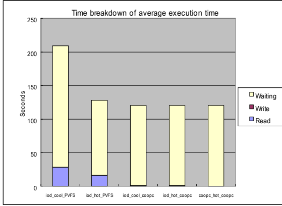
Fig. 3. Execution time breakdown of the matrix multiplication program
